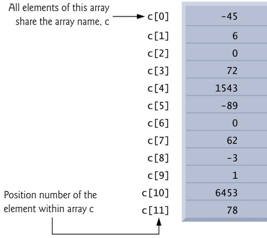
**Fig. 6.1** | 12-element array.
