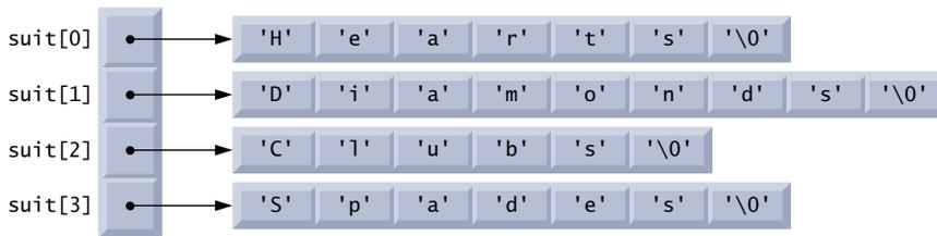
**Fig. 7.22** | Graphical representation of the `suit` array.
