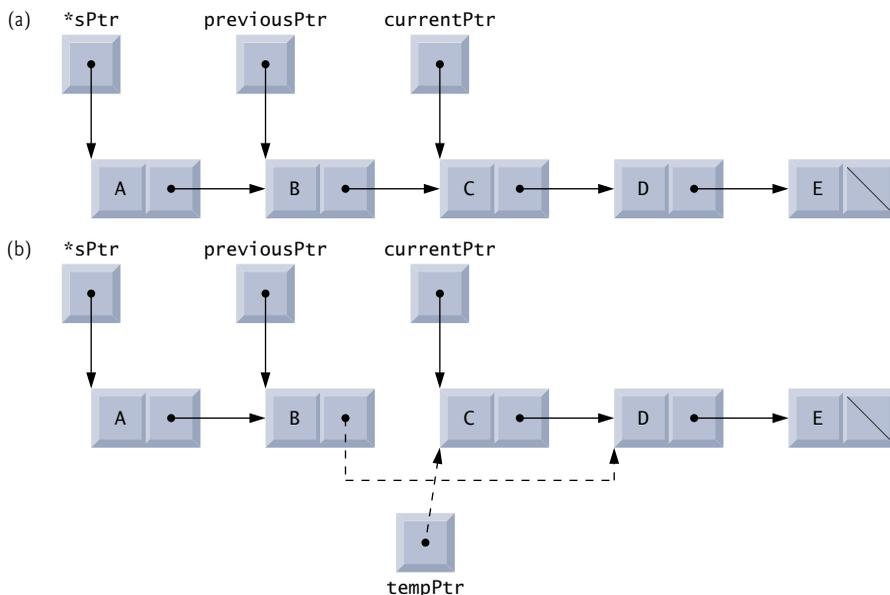
**Fig. 12.6** | Deleting a node from a list.
