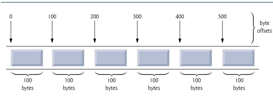
**Fig. 11.9** | C's view of a random-access file.
