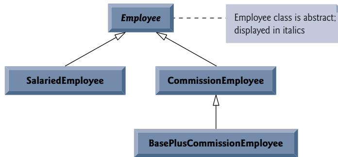
**Fig. 20.7** | Employee hierarchy UML class diagram.
