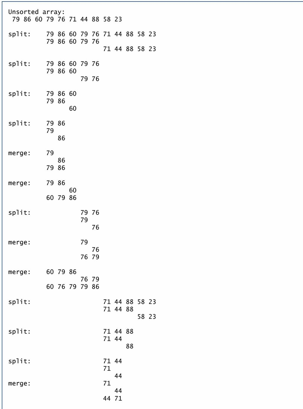
**Fig. D.3** | The merge sort algorithm. (Part 4 of 5.)
