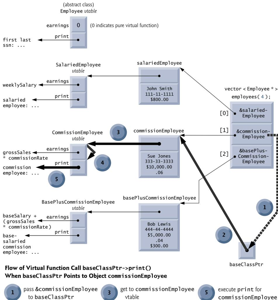
**Fig. 20.18** | How virtual function calls work.
